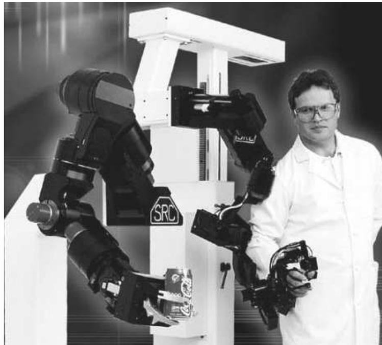
Figure 8.32 : L'exosquelette semi-portable Dextrous Arm Master de Sarcos, copyright photo Sarcos
