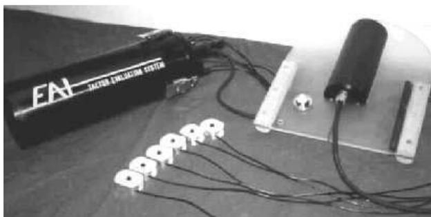
Figure 9.4 : L'interface tactile «Tactor Evaluation System» de Engineering Acoustics, copyright photo Engineering Acoustics
