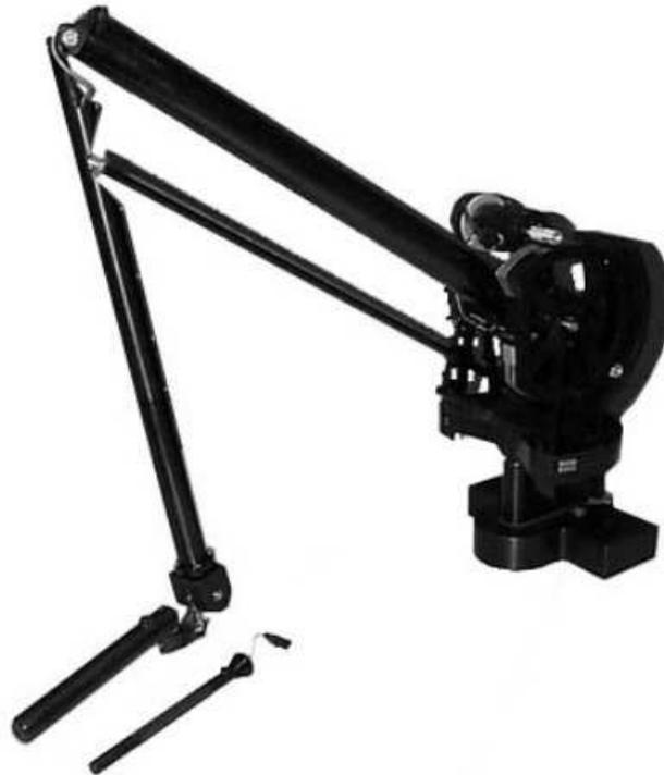
Figure 8.16 : Le Phantom premium, version 3.0 de SensAble, copyright photo SimTeam
