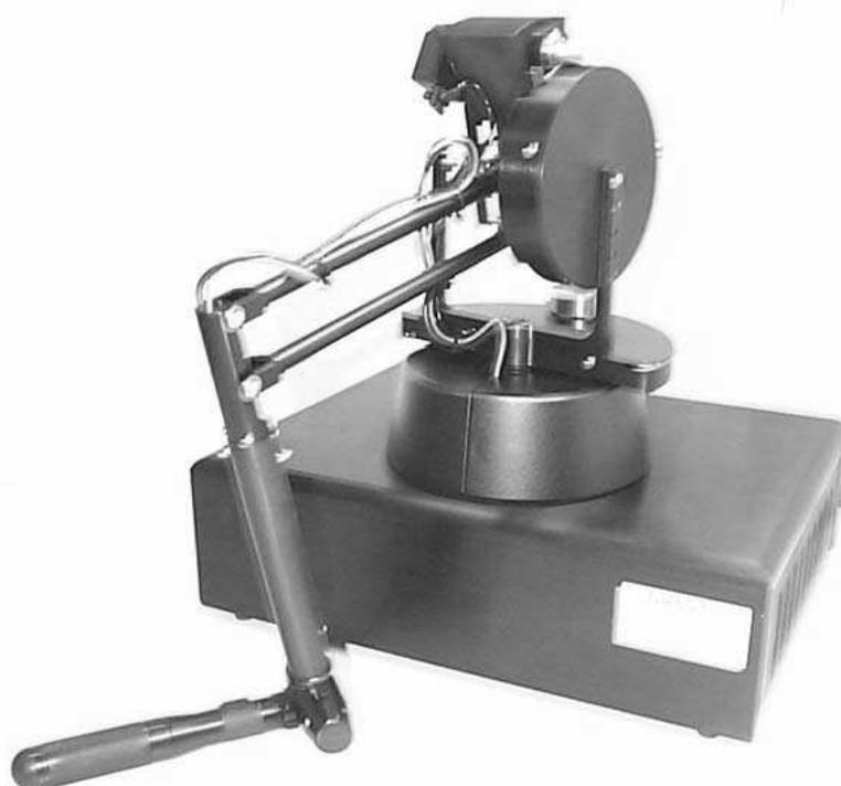
*Figure 8.18 : Le Phantom 1.5/6DOF de SensAble, copyright photo SimTeam*
